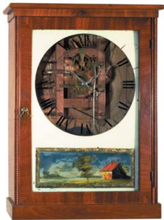
SHELF CLOCK with its revolutionary wooden movement was developed by Eli Terry, a Connecticut clockmaker working in the 19th century. Terry's ingenious mass-production techniques made possible the manufacture of affordable clocks.
