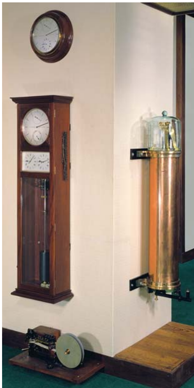
FREE PENDULUM CLOCKS were developed by William H. Shortt, an English railroad engineer, in the early 1920s. Shortt's timekeeping systems, which incorporated two pendulum clocks—a "master" (right) and a "slave" (left)—were reportedly able to keep time to within about a second a year.
